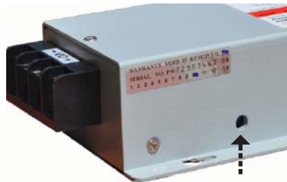
Figure 1: Location of the “right” potentiometer adjustment hole
