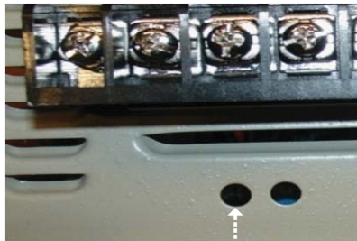
Figure 1: Location of the “Left” potentiometer adjustment hole
